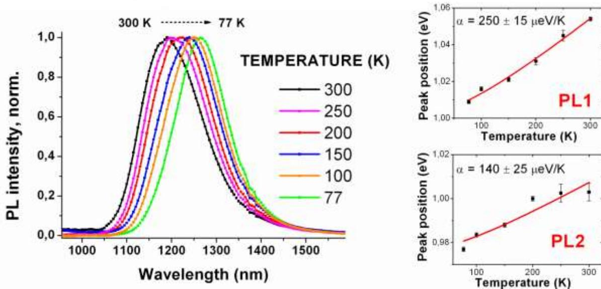
Fig.1. Typical red shift of the PL peak position with temperature decrease, recorded for 4.4 nm PbS QDs. PL spectrum composed of 2 PL components, Varshni fit and estimated temperature coefficients  $\alpha$  of the PL peak position shift for PL1 and PL2 are shown in the right panel.
