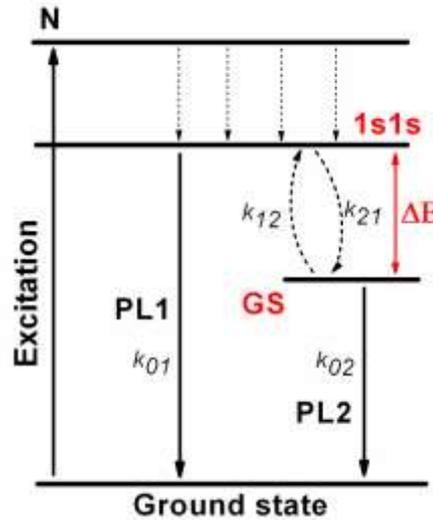
Fig. 2. The scheme of energy relaxation in intermediate -sized PbS QDs: PL1 relates to the 1s1s state and PL2 relates to the in-gap state (GS). Two these radiative states are separated by the  $\Delta E$  energy gap and are coupled by nonradiative transitions  $k_{21}$  and  $k_{12}$ . PL1 and PL2 bands are characterized by recombination rates  $k_{01}$  and  $k_{02}$ , respectively.
