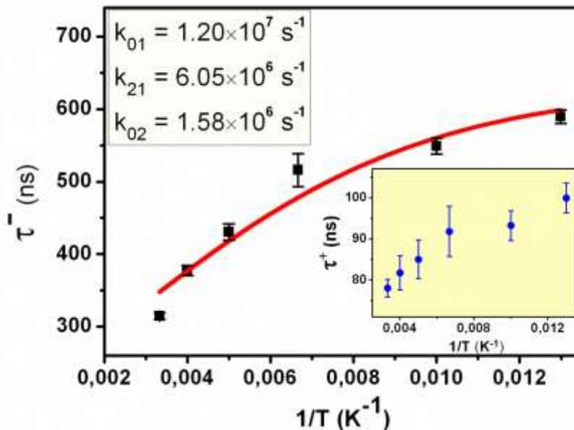
Fig.5. Measured and calculated  $\tau^-$  for 4.4 nm PbS QDs. Inset – measured  $\tau^+$  for 4.4 nm.
