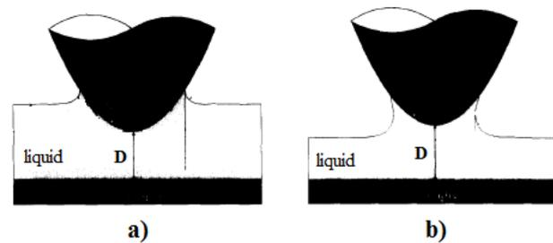
**Fig. 9** The meniscus of the water vapor layer adsorbed on the sample surface onto a paraboloidal tip, during a) approach and b) retraction, where D is the distance from the sample [6]
