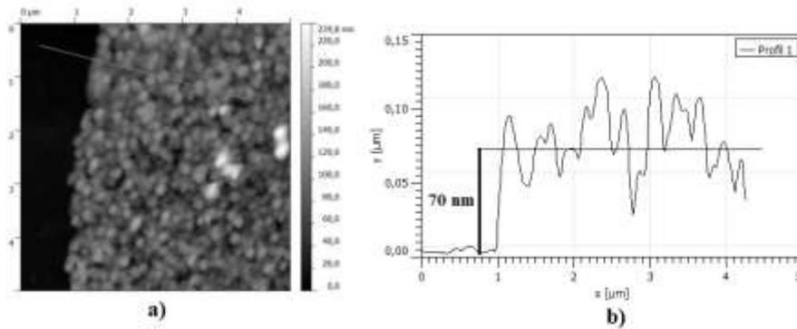
**Fig. 7** AFM image of transition between the layer and glass of PANI\_20, a) 2D image, 5x5μm, b) profile of this step
