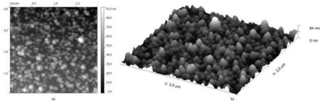
**Fig. 3** AFM image of topography of layer PANI\_10, 5x5 $\mu\text{m}$ , a) 2D, b) 3D
