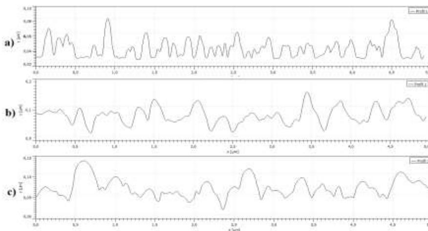
**Fig. 6** The profiles of roughness, a) PANI\_10, b) PANI\_20, c) PANI\_30
