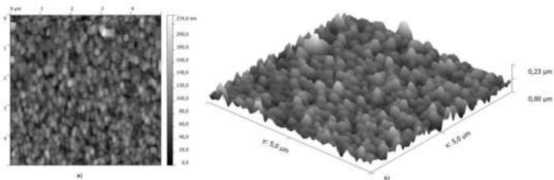
**Fig. 4** AFM image of topography of layer PANI\_20, 5x5 $\mu\text{m}$ , a) 2D, b) 3D
