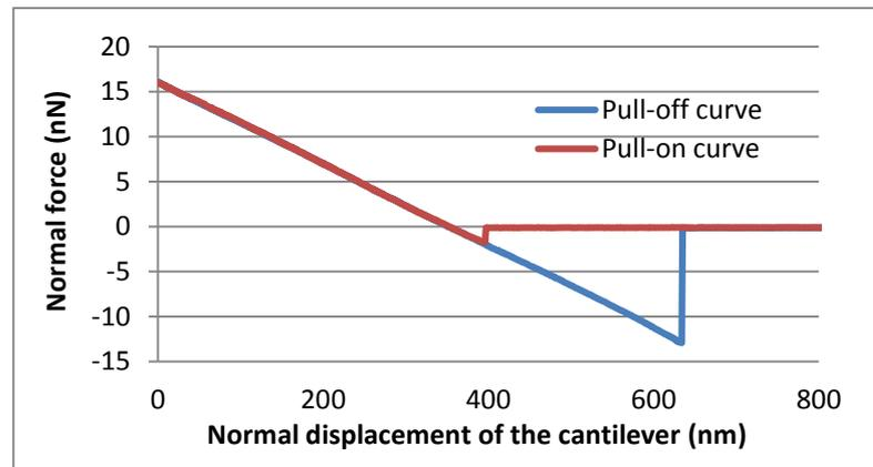
**Fig. 2** Typical adhesion curve for tip with gold coating and layer PANI\_10
