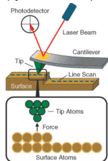
**Fig. 1** Principle of the AFM measurement [2]
