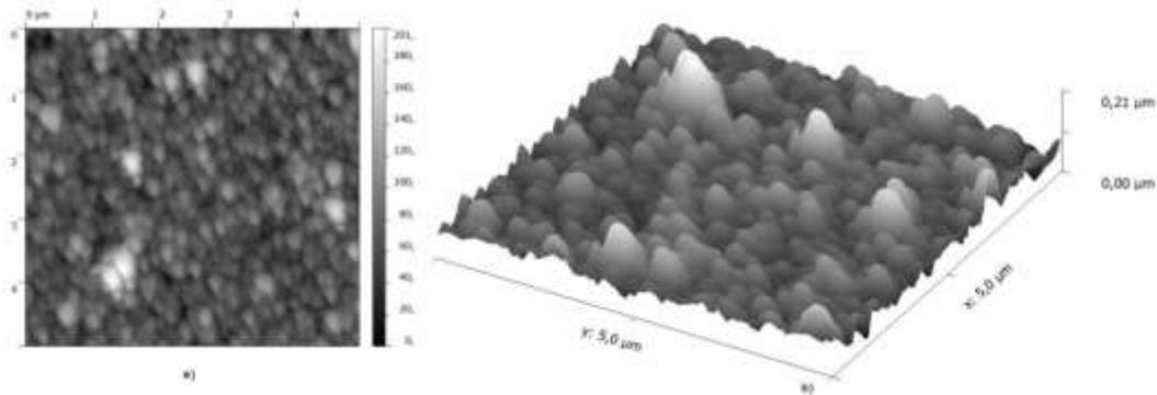
**Fig. 5** AFM image of topography of layer PANI\_30, 4.9x4.9μm, a) 2D, b) 3D
