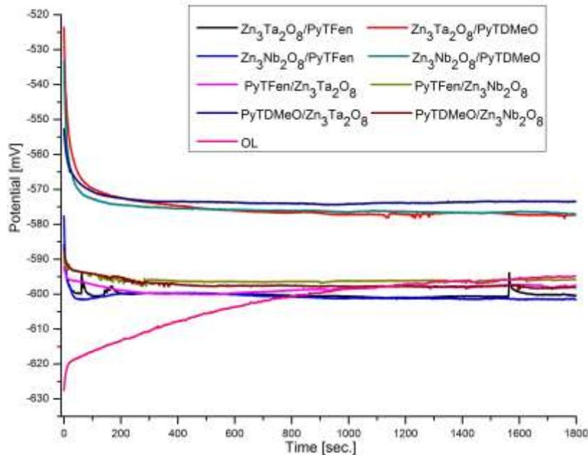
**Fig. 2.** Evolution of OCP with time, in 0.1 mole/L  $H_2SO_4$  electrolyte solution, recorded for bare and bilayer modified carbon steel electrodes:  $Zn_3Ta_2O_8/PyTFen$ ;  $Zn_3Ta_2O_8/PyTDMEO$ ;  $Zn_3Nb_2O_8/PyTFen$ ;  $Zn_3Nb_2O_8/PyTDMEO$ ;  $PyTFen/Zn_3Ta_2O_8$ ;  $PyTFen/Zn_3Nb_2O_8$ ;  $PyTDMEO/Zn_3Ta_2O_8$  and  $PyTDMEO/Zn_3Nb_2O_8$
