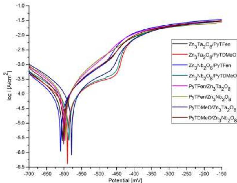
**Fig. 3.** Tafel representation of polarisation curves recorded in 0.1 mole/L  $H_2SO_4$  for the bilayer modified carbon steel electrodes,  $v = 1$  mV/s.
