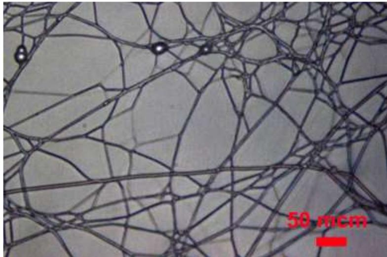
**Fig. 4** Detail of PVA microfiber mat with the encapsulated probiotic bacteria depicted by optical microscopy
