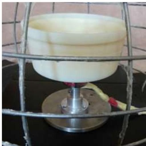
Fig. 1 Polyamide bell for the centrifugal microfiber production
