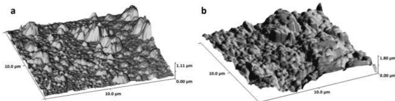
**Fig. 3.** AFM images of (a) PANI/MMT\_10 on left, and (b) PANI/MMT\_20 on right.
