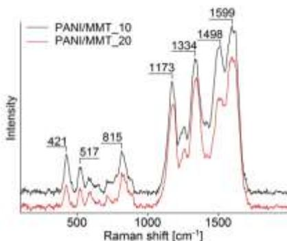
**Fig. 2.** Raman spectra of both PANI/MMT\_10 and PANI/MMT\_20 samples.
