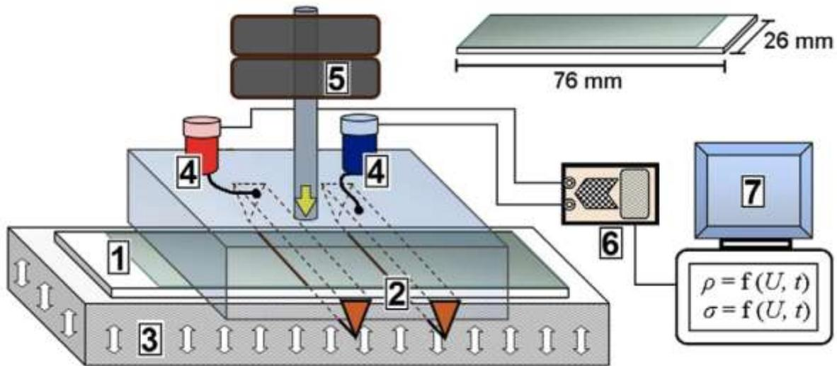
**Fig. 1.** Measuring device of DC conductivity. 1) sample - thin film on glass slide (glass slide dimensions in upper right corner); 2) Cu-electrodes (distance 3 mm); 3) flexible insulator; 4) voltage terminals; 5) weights to provide constant load; 6) measuring card; 7) PC + software
