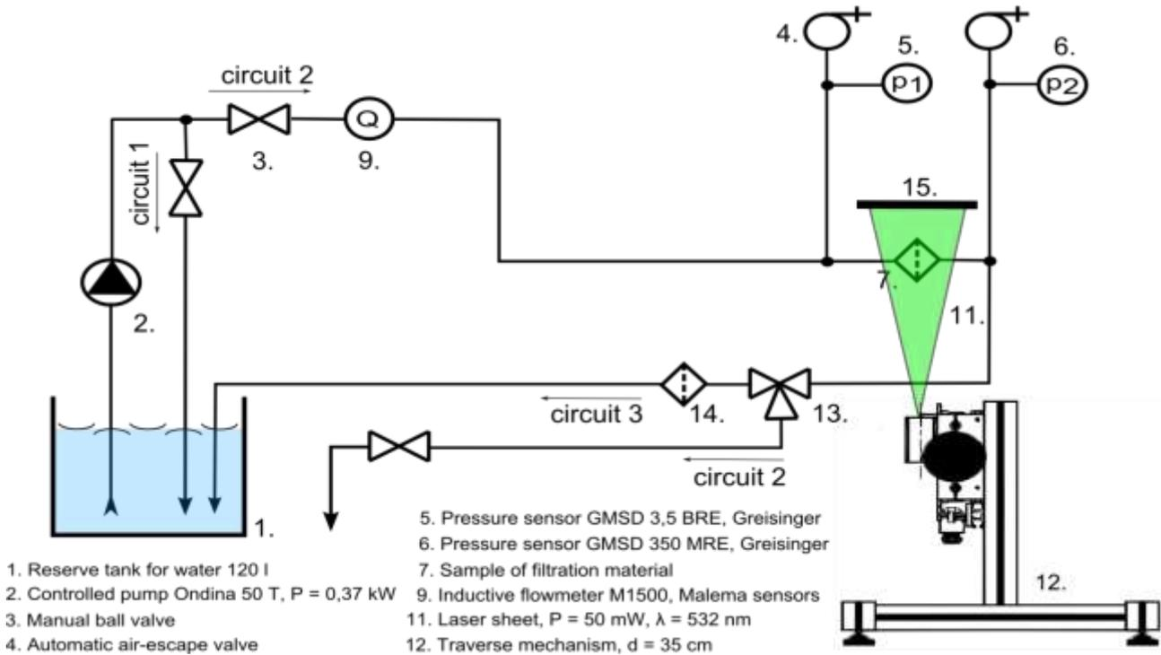
Fig. 1 Scheme of the filtration setup
