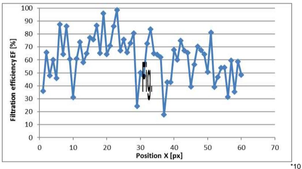
Fig. 9. Filtration efficiency versus position of nanofibrous filtration textile.
