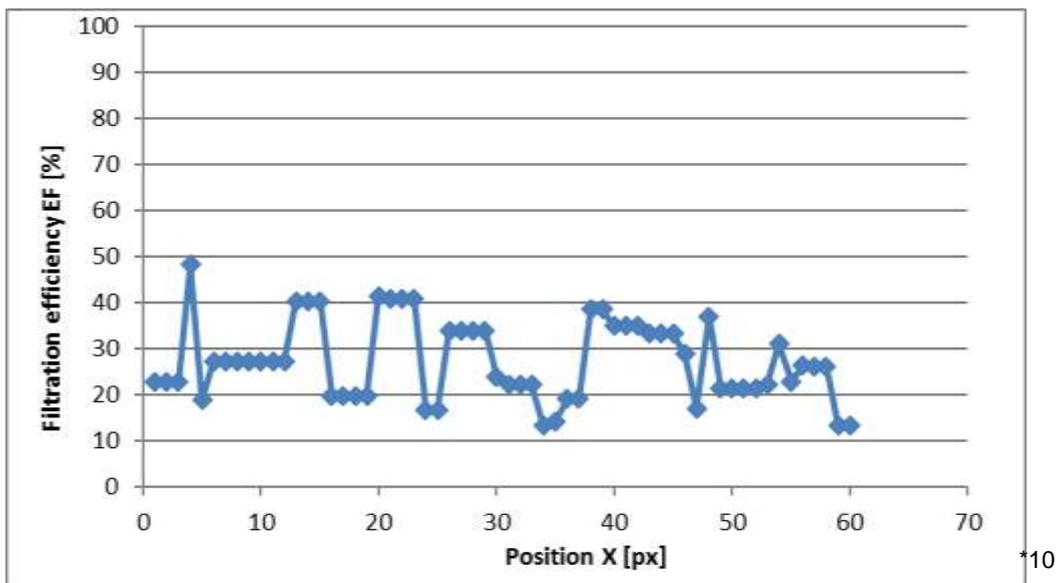
Fig. 8. Filtration efficiency versus position of woven filtration textile.
