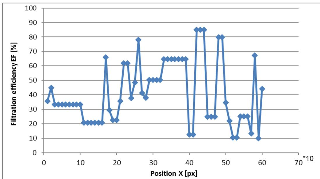
Fig. 7 Filtration efficiency versus position of non-woven filtration textile (meltblown)
