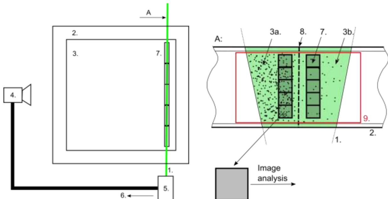
Fig. 6 Block scheme of the measurement principle: 1: laser sheet, 2: filtration channel from glass, 3: water seeded by artificial particles, 3a: upstream, 3b: downstream, 4: camera, 5: laser unit, 6: direction of the traversing, 7: evaluative areas, 8: sample of a filtration textile, 9: an area of flow seen by the camera
