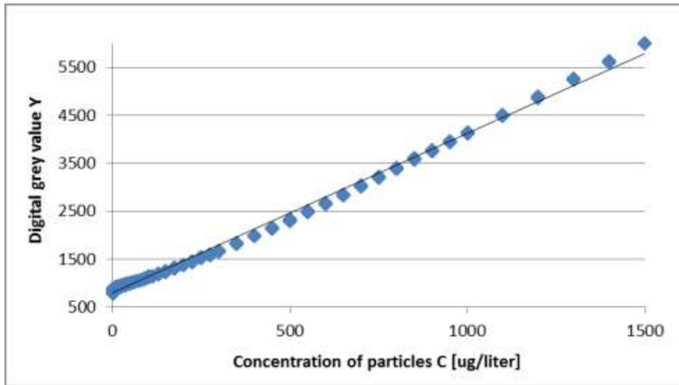
Fig. 5 Curve of digital grey value versus concentration of particles
