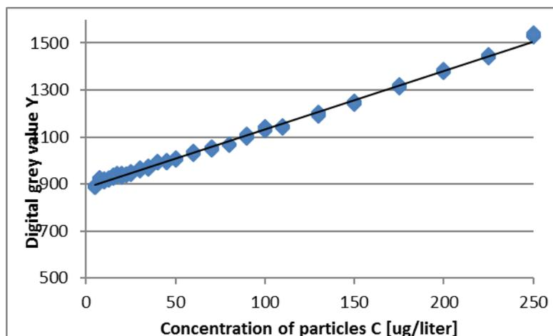
Fig. 4 Curve of digital grey value versus concentration of particles
