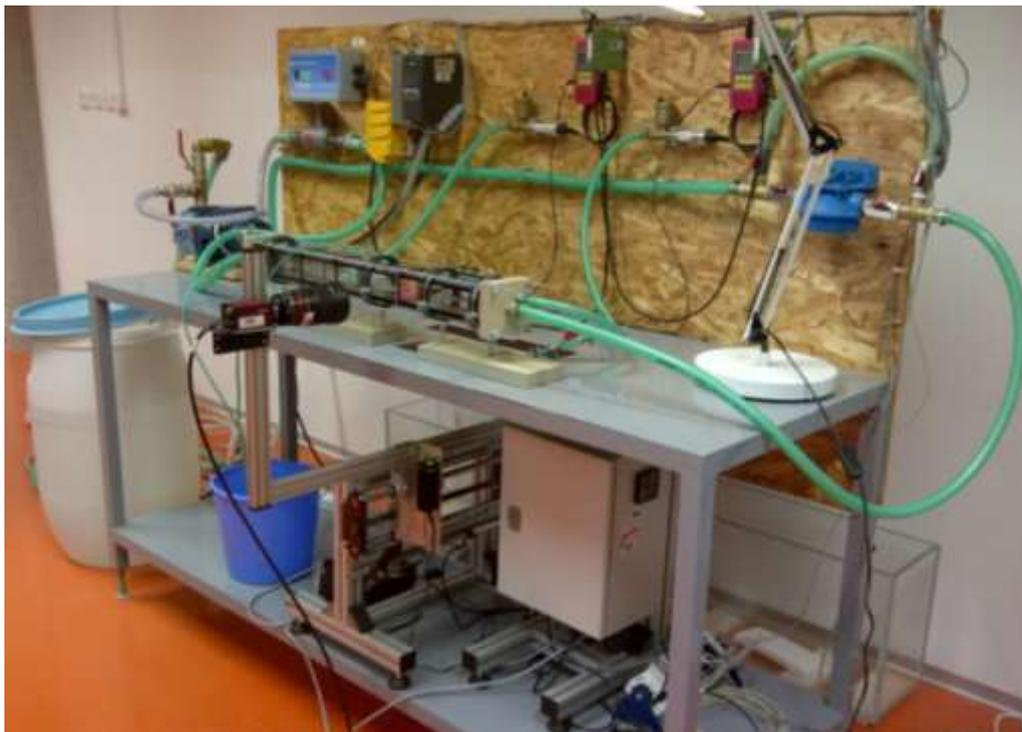
**Fig. 2** Picture of the filtration apparatus in laboratory
