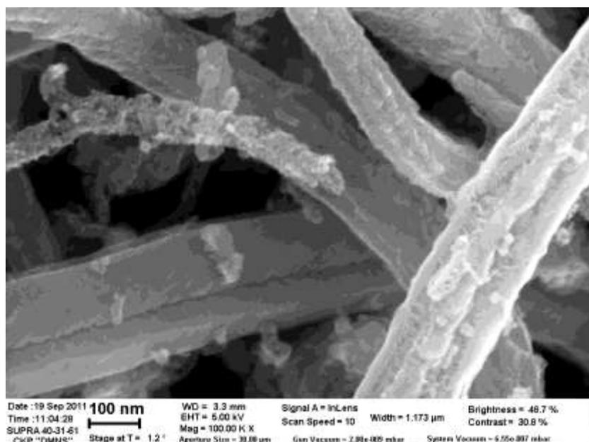
**Fig.3** MWCNTs after the introduction of the nitrophenyl fragments
