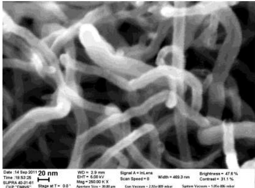
**Fig.2** Non-functionalized MWCNTs
